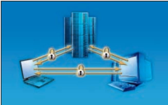
Trusted Clients communicate their platform configuration. Prior to a transaction, other Trusted Clients and Servers use this information to verify the clients are operating in an uncompromised state.
